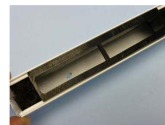
**RECESS FITTING** Option C Drill 3.5 mm holes through the sides of guides, for directly fixing into the recess. Typically two or three depending on height.
