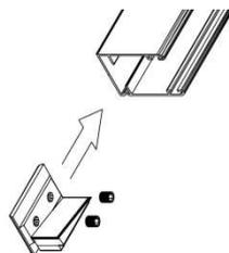
**OPTIONAL INTERMEDIATE STOPS.** If using the optional intermediate stops, slide into the guide ensuring the "wedge" is to the (grooved) front of the side guide. Leave loose, adjust to desired height once the screen has been installed.
