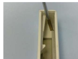
Slide the catches (marked L or R) into the appropriate guide as shown. Ensure the hook is to the (grooved) front. Crimp the guide to hold the catch firmly in place. This prevents catches being forced out in operation.
