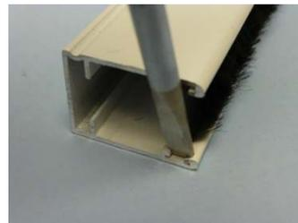
To avoid the fluffy pile being pulled back into the cassette during use. Trim about 6mm off the length of the pile. Simply crimp the channel at each end with a flat headed screwdriver and hammer. *(Tip) Gently does it! Avoid bending the guide out of shape by hitting too hard.*
