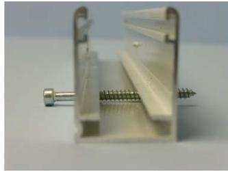
**FACE FITTING** Option A Drill a 3.5 mm hole through the outer groove, ensuring you remain within the recessed area in pic 2.
