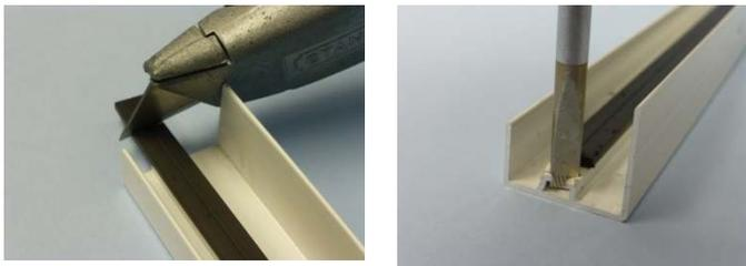
Snip off a small piece of the magnet. Crimp both ends as shown to secure the strip in place.
