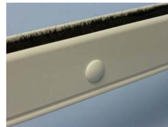
**FACE FITTING** Option B Drill directly through the guide using a 3mm bit. Open up the front facing hole to 7mm and use the cover caps provided for a neat finish.
