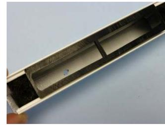
**RECESS FITTING** Option C Drill 3.5 mm holes through the bottom of guides, for directly fixing into the recess. Typically two or three depending on height.
