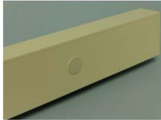
**FACE FITTING** Option A Drill directly through the guide using a 3mm bit. 15mm in from the outer edge. Open the front facing hole to 7mm and use the cover caps provided for a neat finish.
