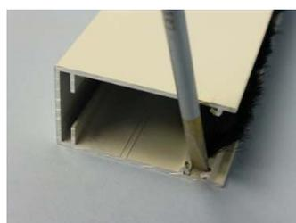
To avoid the fluffy pile being pulled back into the cassette during use. Trim about 6mm off the length of the pile. Simply crimp the channel top and bottom with a flat headed screwdriver and hammer.
