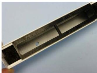
**RECESS FITTING** Option B Drill 3.5 mm holes through the sides of guides, for directly fixing into the recess. Typically two or three depending on height.
