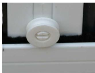
**Attention;** The guide wheel sits on the bottom channel only. This applies to both single and double door models. The screen will not work correctly if fitted "upside" down , and any damage will not be covered under warranty
