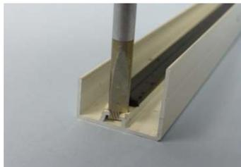
Snip off a small piece of the magnet. Crimp both ends as shown to secure the strip in place.
