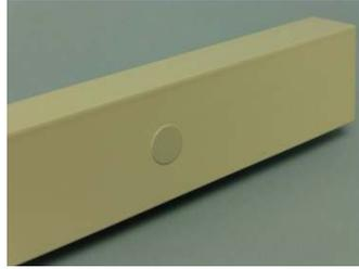
**FACE FITTING** Drill directly through the front and back of the guides using a 3mm bit. **TO AVOID THE PULL BAR FOULING** it is advisable that the holes in the bottom bar are 12mm up from the bottom edge. Alternatively the bottom guide can be affixed using double sided tape. Open the front facing holes to 7mm and use the cover caps provided for a neat finish.
