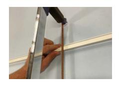
Insert PVC corners into the longest pair of profiles. The corners should be a push fit, but can be gently tapped home with a soft mallet if required. Take note of the spline groove.
